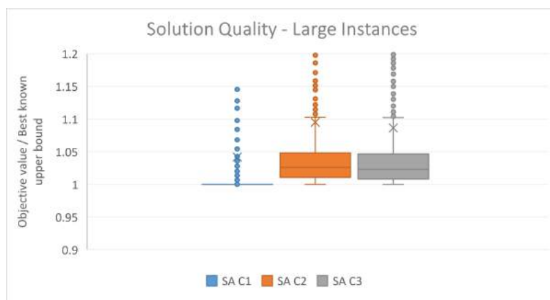
Fig. 6: Box plots comparing the overall results achieved with the simulated annealing approach on the set of larger instances. The vertical axis measures the achieved relative objective values (solution cost produced by each method divided by the overall best found solution cost). Note that some outliers have been excluded for an improved visual comparison.
